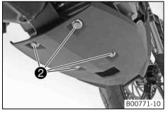
Mount and tighten screws ②.
