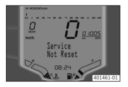
**Service Not Reset** appears on the info display for 10 seconds when the ignition is switched on and the distance interval between service appointments has been exceeded or the service interval display was not reset during a service appointment.
