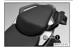
The seat lock **①** is located to the left of the seat. It can be locked with the ignition key.
