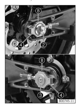
Pull the rear wheel back and mount wheel spindle 3.
