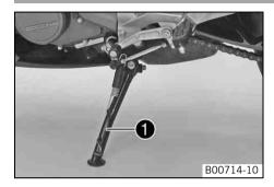
The side stand **1** is on the left side of the vehicle. The side stand is used to park the motorcycle.
