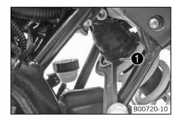
Adjust the spring preload by turning adjustment unit ①.
