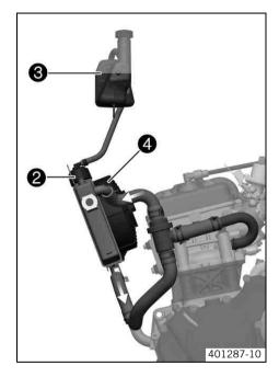
The coolant is cooled by the air stream and a radiator fan  $oldsymbol{4}$ , which is controlled by a thermoswitch.
