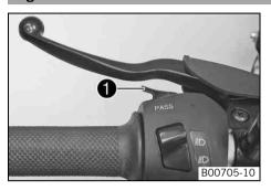
The high beam flasher button • is fitted on the left side of the handlebar.
