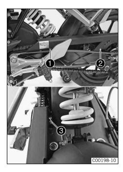
Position the chain guard and tighten screws ①, ②, and ③.
