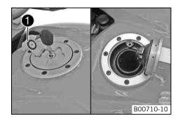
Lift the cover • of the filler cap and insert the ignition key in the lock.
