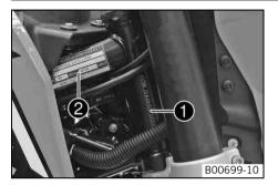
The chassis number **1** is stamped on the right of the steering head. The type label **2** is on the right of the frame behind the steering head.
