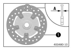
Check the thickness of the front and rear brake discs at several places on the disk to see if it conforms to measurement .
