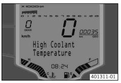
**High Coolant Temperature** appears on the info display if the coolant temperature rises above the specified value.
