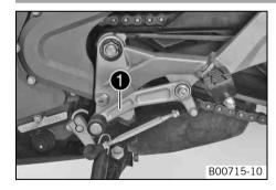
Shift lever **1** is mounted on the left side of the engine.
