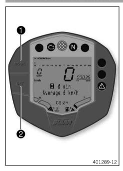
You can change the display mode with the **MODE** button **1**. Possible display modes are total distance traveled (**TRIP 1**), distance 1 (**0D0**) and distance 2 (**TRIP 2**).
