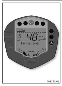
If the fuel level drops to the reserve mark, the display mode automatically changes to **TRIP F** and starts to count from **0.0**, regardless of the previous display mode.
