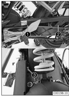
Remove screws 2 and 3 and release screw 1. Push the chain guard aside.
