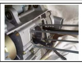
Clean the residues attached onto the matching surfaces of cylinder and crankcase.
