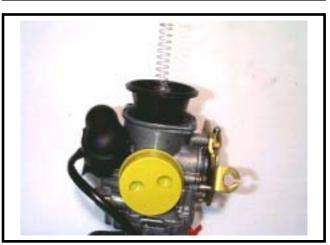
Install vacuum chamber cover and tighten 2 screws.
