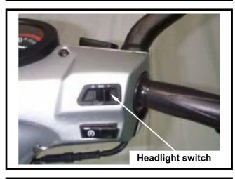
High/Low beam switch & Passing switch
