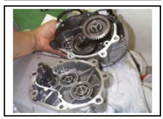
Install new driving shaft bearing into left crankcase.
