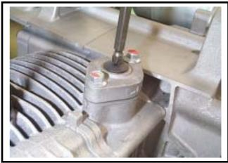
Remove the cam sprocket. (bolt x2)
