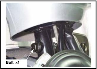
Remove the handlebar assembly.
