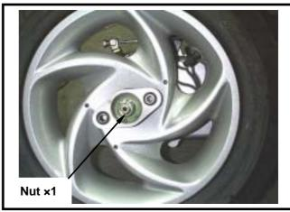
Remove the rear brake adjustment nut.
