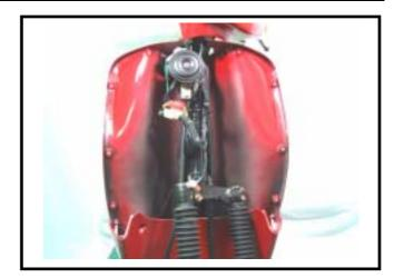
Remove the power coupler of the meter.
