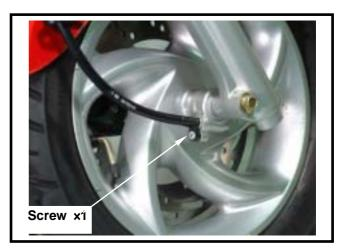
Remove the front fender screws. (left & right x 2)
