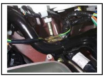
Remove the winker relay coupler.
