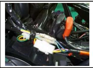
Remove the starter motor cable on the relay.
