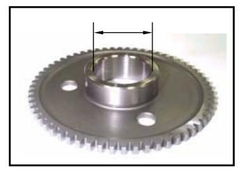
Check the starting idle gear and shaft for wear or damage.
