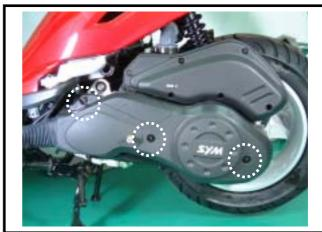
Loosen the clamp of the engine left cover air duct, and then remove the duct.
