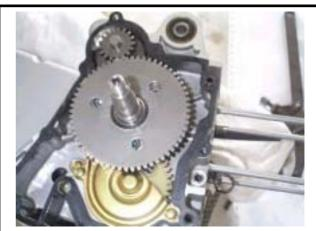
Remove starting clutch, starting idle-gear, and shaft.
