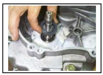
Press-fit the oil seal to specified position with the oil seal installer (25x37x6). Special service tools: the oil seal installer
