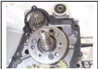
Install the starting driven gear onto the starting clutch.
