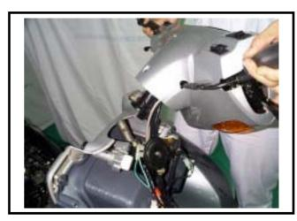
Remove the main switch connector and bolts. (bolts x 3)
