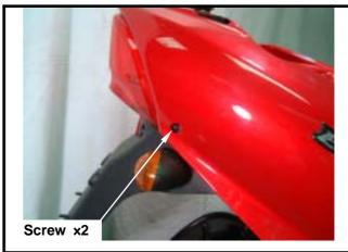
Remove the seat lock cable, then remove the body cover.
