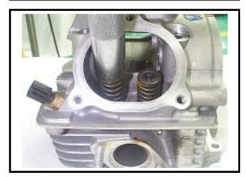
Tap valve stem to make valve retainer and valve stem sealing properly.
