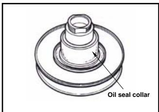
Remove guide pin, guide pin roller, and sliding driven face, and then remove O-ring & oil seal seat from sliding pulley.
