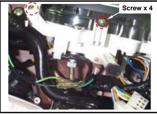
Disassemble the instrument seat and the instrument. (screw x 2)
