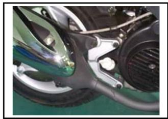
Remove the cooling fan. (4 bolts)
