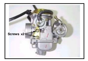
Remove the screws (screw x 2) of the air cut-off valve and its cover.
