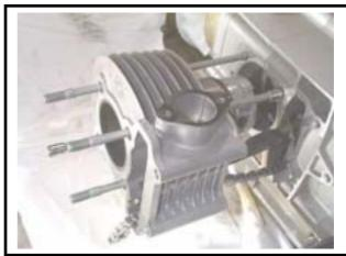
Remove cylinder gasket and lock pins.
