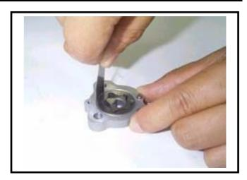
Check clearance between inner and outer rotors.
