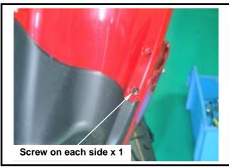
Remove 2 screws on the left & right each side of side cover.
