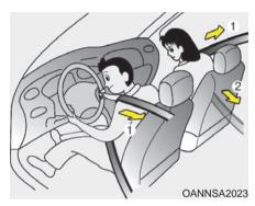
Your vehicle is equipped with pre-tensioner seatbelts in the front seating positions (driver side with retractor pre-tensioner, passenger side with retractor and EFD (Emergency Fastening Device)).
