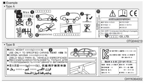
\* The actual Jack label in the vehicle may differ from the illustration. For more detailed specifications, refer to the label attached to the jack.
