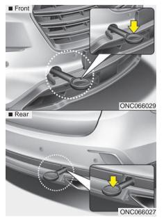
If towing is necessary, we recommend you to have it done by an authorized HYUNDAI dealer or a commercial tow truck service. If towing service is not available in an emergency, your vehicle may be temporarily towed using a cable or chain secured to the emergency towing hook attached to the front (or under the rear) of the vehicle.
