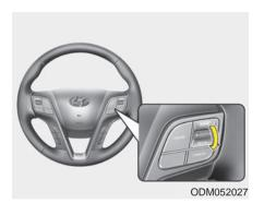
3. Push the toggle switch down (SET-), and release it at the desired speed.
