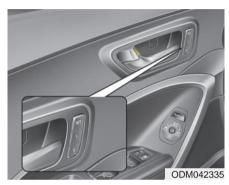
A driver position memory system is provided to store and recall the driver seat and side view mirror position with a simple button operation. By saving the desired position into the system memory, different drivers can reposition the driver seat based upon their driving preference. If the battery is disconnected, the position memory will be erased and the driving position should be restored in the system.
