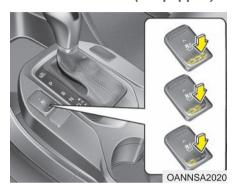
The air ventilation seat is provided to cool the front seats during hot weather by blowing air through small vent holes on the surface of the seats. While the engine is running, press the cooling portion (blue color) of the switch to cool the driver's seat or the front passenger's seat.
