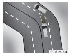
While driving on a curve, the AEB may recognize a vehicle in front the next lane over. Exercise caution, and, if necessary, depress the brake pedal.
