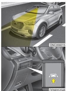
This system detects the lane with the sensor at the front windshield and warns you when your vehicle leaves the lane.
