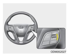
3. Move the toggle switch down (to SET-), and release it at the desired speed. The SET indicator light in the instrument cluster will illuminate. Release the accelerator pedal at the same time. The desired speed will automatically be maintained.
