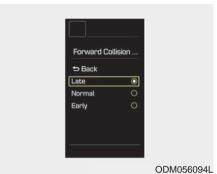
The driver can set the alarm speed to Early, Normal, or Late by placing the ignition switch to the ON position and by selecting 'User Settings', 'Driving Assist', 'FCW (Forward Collision Warning)', and 'Early / Normal / Late'
