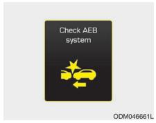
This warning message illuminates if there is a malfunction with the Automatic Emergency Braking (AEB) system, have your vehicle inspected by an authorized HYUNDAI dealer.
