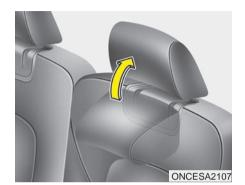
Unfold the headrest - 3rd row To unfold the headrest : Raise the headrest manually.
