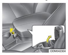
To open the center console storage, pull up the lever.
