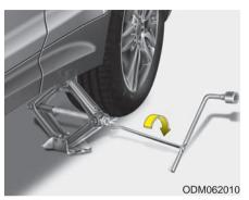
8. Insert the jack handle into the jack and turn it clockwise, raising the vehicle until the tire just clears the ground. This measurement is approximately 1.2 in (30 mm). Before removing the wheel lug nuts, make sure the vehicle is stable and that there is no chance for movement or slippage.
