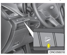
The Downhill Brake Control (DBC) assists the driver when descending a steep hill without the driver depressing the brake pedal. It slows the vehicle to approximately 6.3 mph (10 km/h) and lets the driver concentrate on steering the vehicle.
