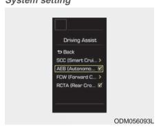
The driver can activate the AEB by placing the ignition switch to the ON position and by selecting 'User Settings', 'Driving Assist', and 'AEB (Automatic Braking System)'. The AEB deactivates, when the driver cancels the system setting.
