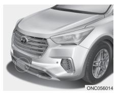
The sensor is to maintain a certain distance from the vehicle in front. However, a smudged sensor lens with foreign substances, such as snow and rain, adversely affects the sensing performance. It may even temporarily cancel the AEB. Always keep the sensor lens clean.
