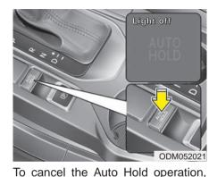
press the Auto Hold switch. The AUTO HOLD indicator will disappear. To cancel the Auto Hold operation when the vehicle is at a standstill, press the Auto Hold switch while depressing the brake pedal.
