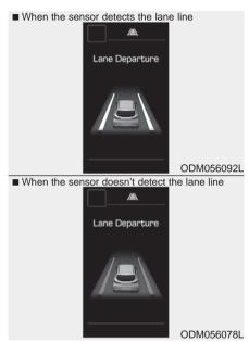
If your vehicle leaves the lane when the LDWS is operating and vehicle speed exceeds 35 mph (60 km/h), the warning operates as follows:
