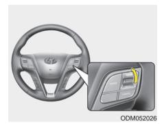
If any method other than the CRUISE button was used to cancel cruising speed and the system is still activated, the most recent set speed will automatically resume when you move the toggle switch up (to RES+). It will not resume, however, if the vehicle speed has dropped below approximately 25 mph (40 km/h).
