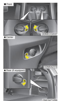
The power outlet is designed to provide power for mobile telephones or other devices designed to operate with vehicle electrical systems. The devices should draw less than 10 amps with the engine running.
