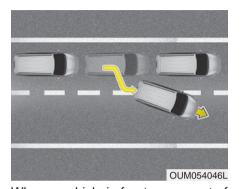
When a vehicle in front moves out of the lane to avoid a stopped vehicle further ahead, the AEB may not detect the stopped vehicle ahead. Always exercise caution.
