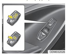
The seat warmer is provided to warm the rear seats during cold weather. With the ignition switch in the ON position, push either of the switches to warm the rear seats.
