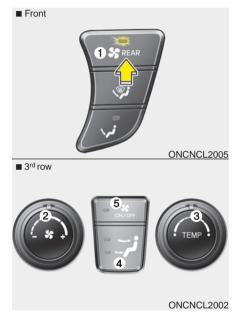
1. To turn the 3<sup>rd</sup> row climate control on or off, press the 3<sup>rd</sup> row climate control ON/OFF button (1 or 5).
