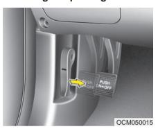
Check whether the stroke is within the recommended specification when the parking brake pedal is fully engaged. When engaged, the parking brake alone should hold the vehicle securely. If the stroke is more or less than specified, have the parking brake adjusted by an authorized HYUNDAI dealer.
