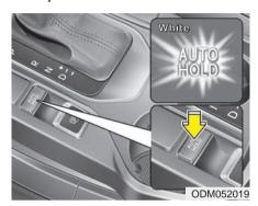
1. With the driver's door, engine hood and liftgate (tailgate) closed, fasten the driver's seat belt or depress the brake pedal and then press the Auto Hold button. The white AUTO HOLD indicator will come on and the system will be in the standby position.
