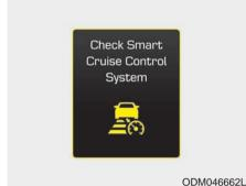
This warning message illuminates if there is a malfunction with the advanced smart cruise control system, have your vehicle inspected
