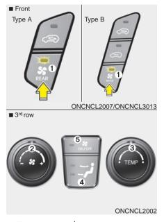
1. To turn the 3<sup>rd</sup> row climate control on or off, press the 3<sup>rd</sup> row climate control ON/OFF button (1 or 5).
