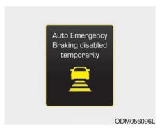
When the sensor cover or the sensor lens is obscured by foreign substances, such as snow or rain, the AEB operation may temporarily stop working. In this case, a warning message will appear to notify the driver. This is not a malfunction with the AEB. To operate the AEB again, remove the foreign substances.
