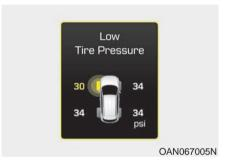
When the tire pressure monitoring system warning indicators are illuminated and warning massage displayed on the cluster LCD display, one or more of your tires is significantly under-inflated. The low tire pressure position telltale light will indicate which tire is significantly under-inflated by illuminating the corresponding position light.
