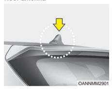
Your vehicle uses a roof antenna to receive both AM and FM broadcast signals.
