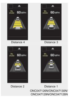
Your vehicle speed will slow down or speed up to maintain the selected distance (A vehicle will appear in front of your vehicle in the LCD display only when there is an actual vehicle in front of you.).  If the vehicle ahead speeds up, your vehicle will travel at a steady cruising speed after accelerating to the set speed.
