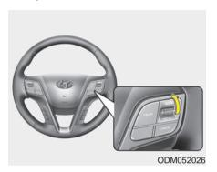
If any method other than the CRUISE toggle switch was used to cancel cruising speed and the system is still activated, the cruising speed will automatically resume when you push the toggle switch up (RES+) or down (SET-).
