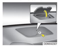
To open the cover, push the lever (1) and the multi box will open automatically.
