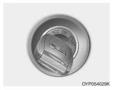
The steering wheel locks to protect against theft. The ignition key can be removed only in the LOCK position. When turning the ignition switch to the LOCK position, push the key inward at the ACC position and turn the key toward the LOCK position.
