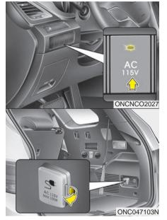
The AC inverter supplies 115V/150W electric power to operate electric accessories or equipments.
