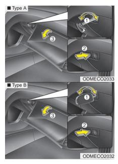
The glove box can be locked and unlocked with the mechanical key (1). To open the glove box, push the button (2) and the glove box will automatically open (3). Close the glove box after use.
