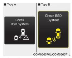
If there is a problem with the BSD system, a warning message will appear and the light on the switch will turn off. The system will turn off automatically. You have your vehicle inspected by an authorized HYUNDAI dealer.
