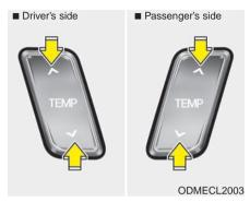
The temperature will increase by pushing the up button. Each push of the button will cause the temperature to increase by 1°F/0.5°C.
