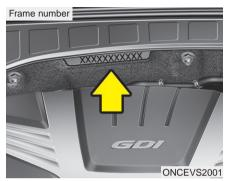
The vehicle identification number (VIN) is the number used in registering your vehicle and in all legal matters pertaining to its ownership, etc. The number is punched on the engine compartment bulkhead.
