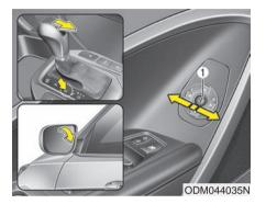
When you shift the shift lever to the R (Reverse) position, the side view mirror(s) will move downward to aid reverse parking.
