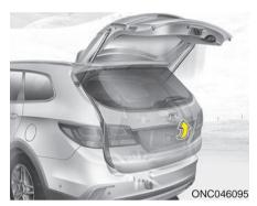
During power opening and closing if the power liftgate (power tailgate) is blocked by an object or part of the body, the power liftgate (power tailgate) will detect the resistance.
