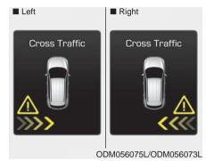
If the vehicle detected by the sensors approaches your vehicle, the warning chime will sound, the warning light on the side view mirror will blink and a message will appear on the LCD display.
