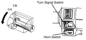
(6). Turn the ignition switch key to the "ON" position, and press horn button down, if the horn does not sound, the fuse may have been blown.
