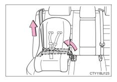
5 If the child restraint has a top tether strap, the top tether strap should be latched onto the top tether strap anchor. (→P. 63)
