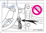
Do not hang coat hangers or other hard objects on the coat hooks. All of these items could become projectiles and may cause death or serious injury, should the SRS curtain shield airbags deploy.
