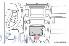
2 Open the cover and connect an iPod using an iPod cable.
