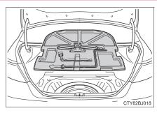
4 Loosen the center fastener that secures the spare tire.
