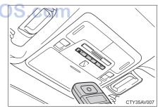
2 Press and hold one of the HomeLink® buttons and the transmitter button. When the HomeLink® indicator light changes from a slow to a rapid flash, you can release both buttons.
