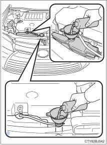
6 Start the engine and turn the air conditioning system on to check that the radiator cooling fans operate and to check for coolant leaks from the radiator or hoses.
