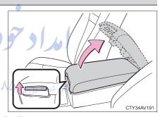
• When using the console box lid as an armrest, slide the console box lid forward as needed. Slide the lid forward while pulling up the lever.
