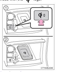
When placing the mobile device on the wireless charging surface of the tray, make sure that there are no objects in-between the mobile device and the tray. They may interfere with charging.
