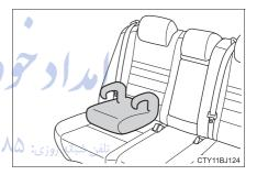
2 Sit the child in the child restraint system. Fit the seat belt to the child restraint system according to the manufacturer's instructions and insert the plate into the buckle. Make sure that the belt is not twisted.
