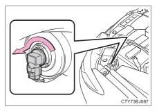
2 Pull the bulb out while pressing the lock release of the connector.
