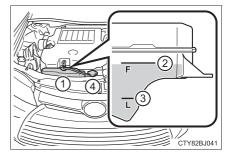
5 Add engine coolant if necessary.
