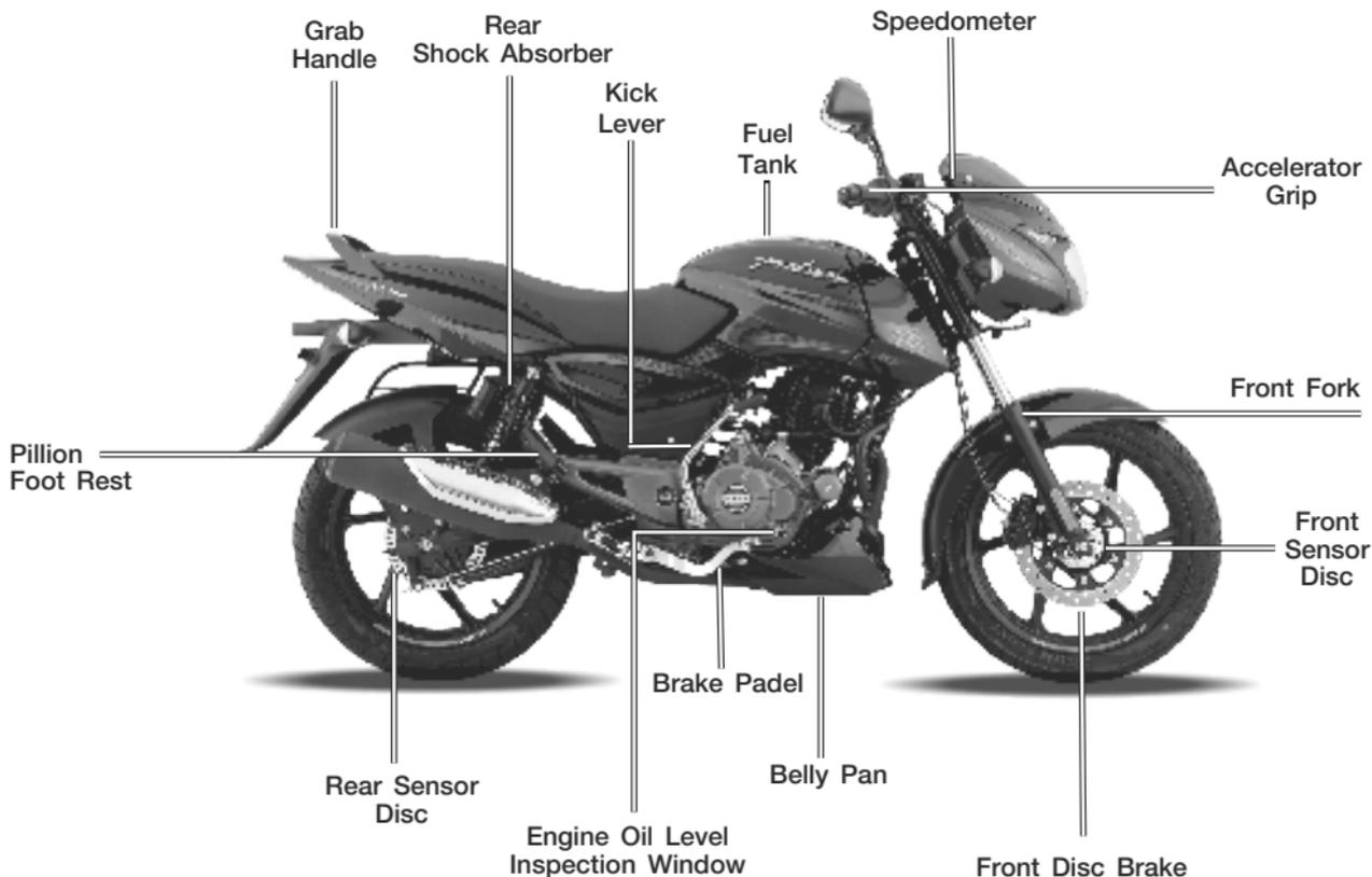
Photograph is of Pulsar 150 Disc-Drum Vehicle
