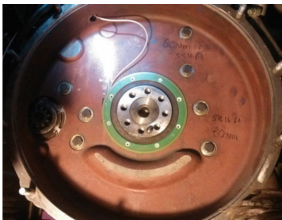
Fig. 4 Installation positions of the stator
