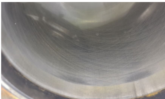
Fig. 25 Reticulate pattern of cylinder
