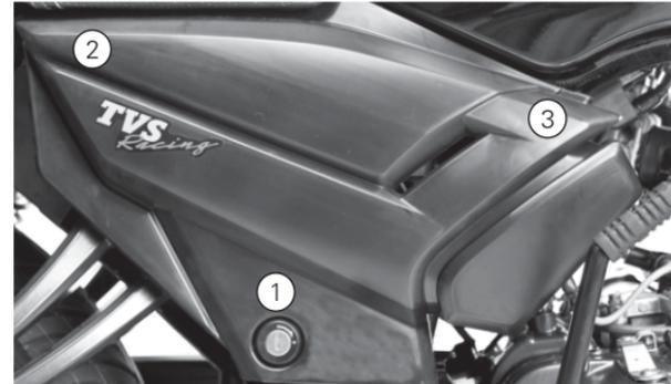
Apache RTR 180 is provided with lockable cover frame on the right side for accessing the battery, rear disc brake master cylinder and the seat lock cable. This cover can be opened in the following manner:
